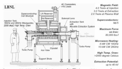
Early test at 28 GHz yielded  $\geq$  8 p $\mu$ A of Bi<sup>30+</sup> ions,  $\sim$ RIA specs for 400 kW Figure 4.1. The ion source developed for RIA . It has delivered 8x10<sup>12</sup> of Bi in charge state +30.
