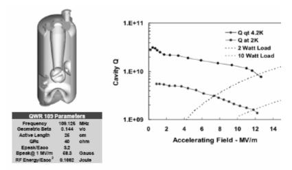
Figure 4.2. Shows the design and performance of a prototype superconducting quarter wave resonator.
