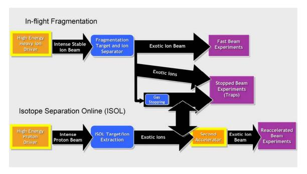
Figure 1.5. Cartoon of the different techniques for creating and utilizing beams of rare-isotopes. The purple boxes represent the final stage where the nuclei are ready for use in experiments.
