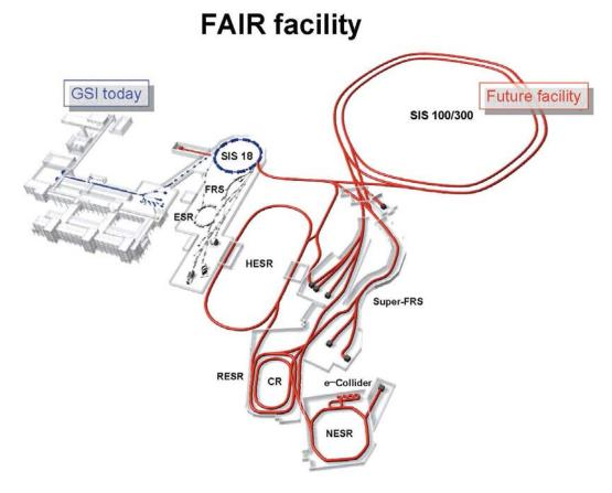
Figure 3.3. Layout of the FAIR facilities. The new accelerators and buildings (indicated in color on the right in the site map) are located east of the existing GSI facilities (indicated in grey).
